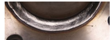
Stainless steel MIG flux-cored wire Current: 270A Voltage: 27.7V
