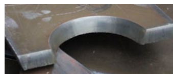
Carbon steel Cutting current: 260A
