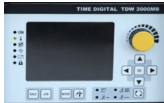
Stainless steel Pulse TIG Base current: 50A Peak current: 100A
